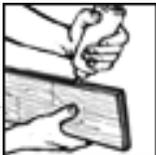
of glue in the *inside bottom edge* of the END groove. DO NOT apply glue to the long side groove at this time Carefully interlock the
